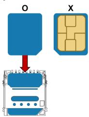
4. Put the holder down and slide it down to lock the holder
