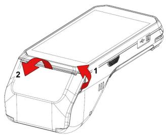
3. Referring to **Figure 19**, put the paper roll into the printer in the correct orientation. The end of the paper roll should be a little unrolled
