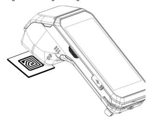
For triggering the RFID read action, press left or right scan button on the PM500 or tap **Read RFID Tag** on the **RFID Demo**.
