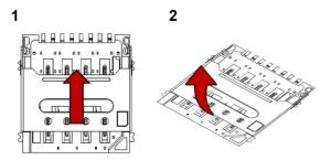
3. Facing down the gold contact of the cards, put the cards in the correct orientation.
