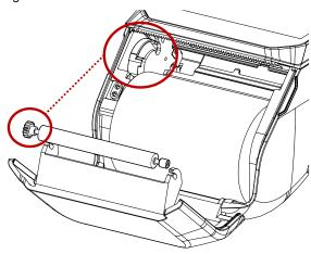
3. Until it clicks, push the both side of the roller firmly in the marked direction in **Figure 23** Figure 23 Reassembled printer roller
