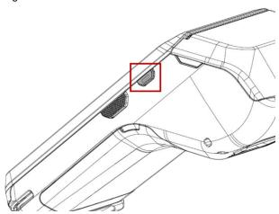
2. When **SMART BEYOND RUGGED** logo displays on the screen, release the button and wait until PM500 finish booting
