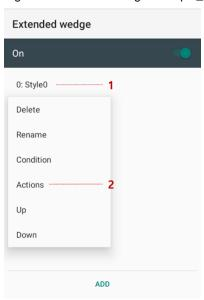
4. Tap ADD and select Move to start to point the start of the decoded data. And then, add another action of which action type is Send string and set value as "Point Mobile". Now you can get decoded data with "Point Mobile" text
